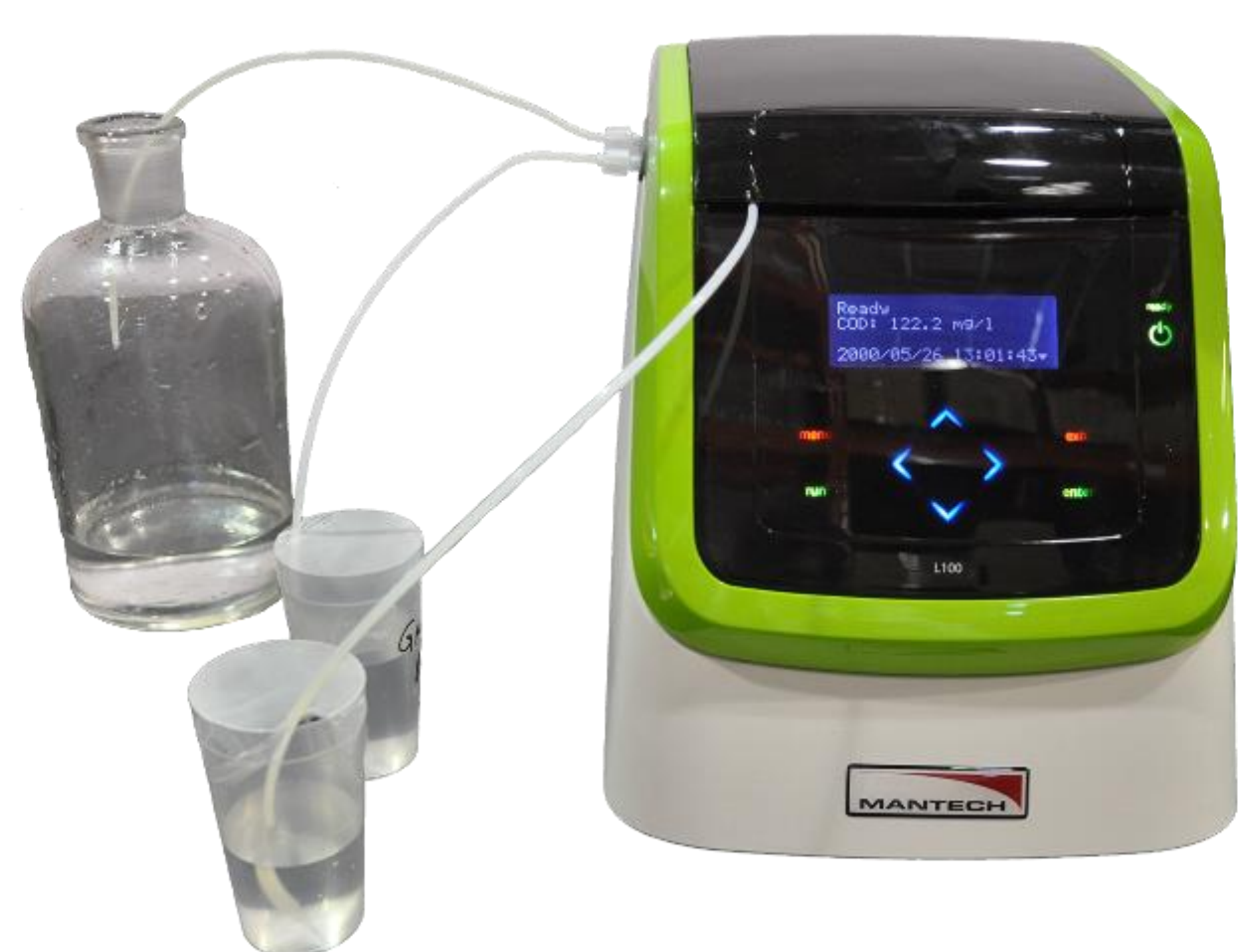
Figure 1. Stand alone PeCOD Unit with sample port, blank port, and waste port.
