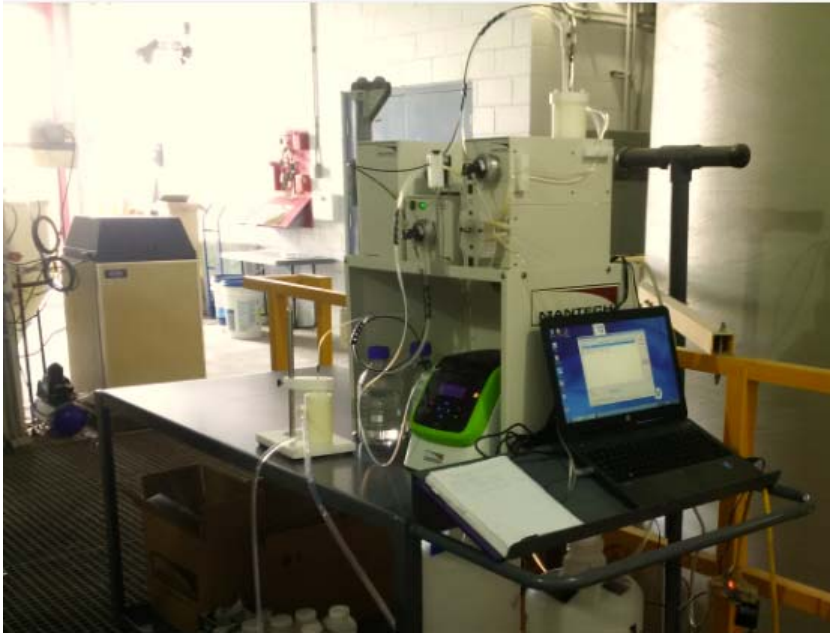
FIGURE 2: AT-LINE L100 PECOD ® LOCATED AT CLARKSON WWTP FINAL EFFLUENT IN MISSISSAUGA, ONTARIO. THE CBOD SAMPLER LOCATED BESIDE THE UNIT (FEATURED TO THE LEFT).
