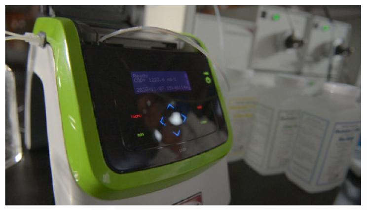
Mantech's PeCOD<sup>®</sup> unit, installed in three food and beverage facilities to explore the feasibility of real-time COD monitoring
