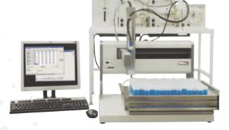
As easy as two clicks of the mouse to operate, TitraSip  $SA^{\mathbb{N}}$  may be configured with or without an autosampler, depending on the number of samples you process. Connect directly to stream analysis for scheduled, operator-independent, multi-parameter analysis.
