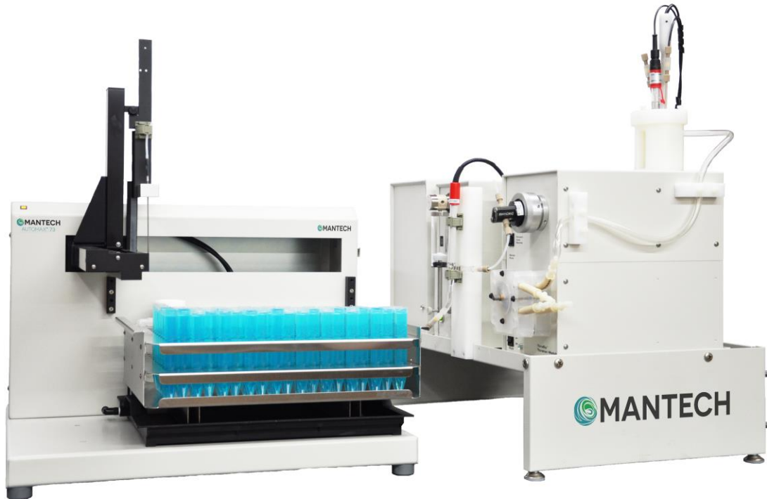
Multiparameter system with one TitraSip™. Analyzes pH, conductivity, alkalinity, fluoride and turbidity from a single sample.
