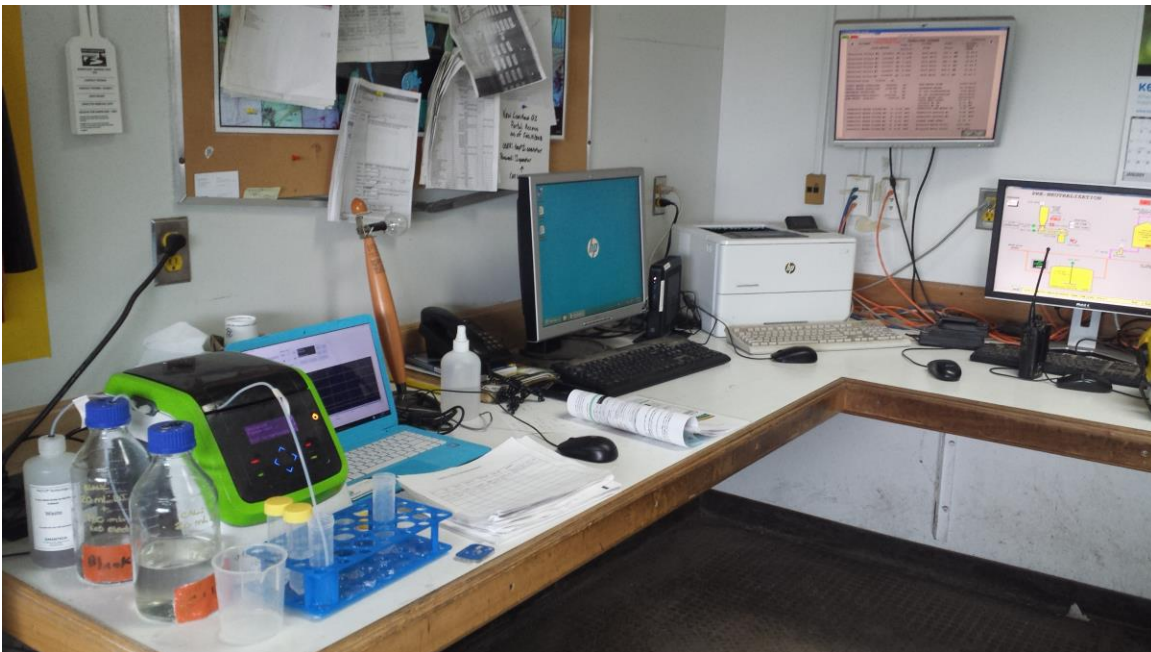
Figure 2: Benchtop PeCOD® COD Analyzer within the secondary treatment facility. The safer technology allows operators to run the test within their office without personal protective equipment (PPE).
