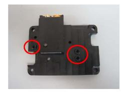
3. Peel off the tape that seals the other end of the internal channel on the other side of the Electrode Block.
