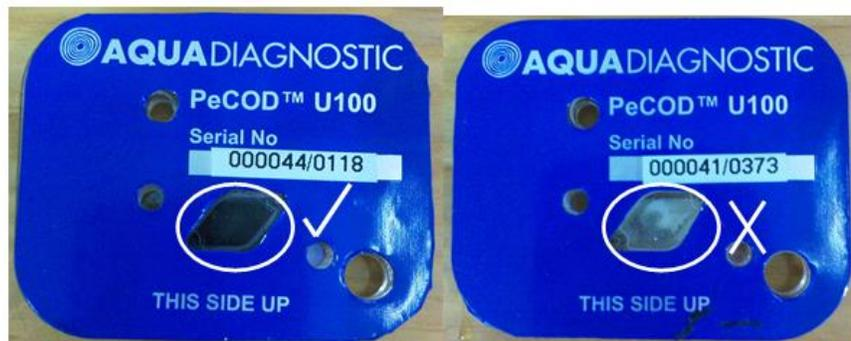
Additionally, if a sensor has lost much of its color, while it may still result in passing M and C calibration values, it may indicate a loss in chloride tolerance. For more information about chloride protection see Technical Bulletin #2011-16.
