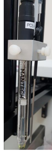
Probe Holder with Fixed Needle at Specific Height
