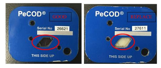
Additionally, if a sensor has lost much of its color, while it may still result in passing M and C calibration values, it may indicate a loss in chloride tolerance. For more information about chloride protection see Technical Bulletin #2011-16.
