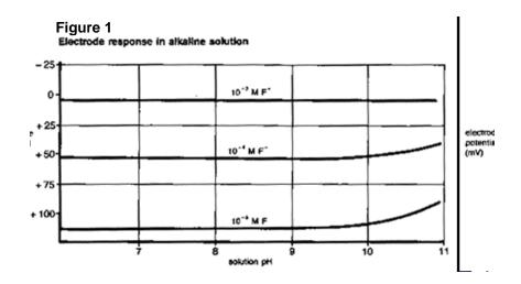
The addition of TISAB 1 or TISAB 2 to all fluoride samples and standards buffers the pH between 5.0-5.5 to help avoid hydroxide interferences or the formation of hydrogen complexes of fluoride. TISAB 3 adjusts the pH to about 8.5 and should not be used for very low level measurements.
