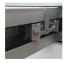
4. Slide the z-arm into the autosampler bracket and tighten the screw once the z-arm height is at 200mm. (If a different z-height is specified on the z-arm, secure the z-arm at the height as marked.)
