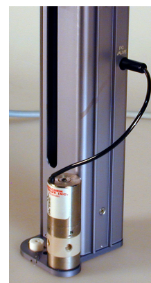
Figure 2-19: FC Valve Installed
