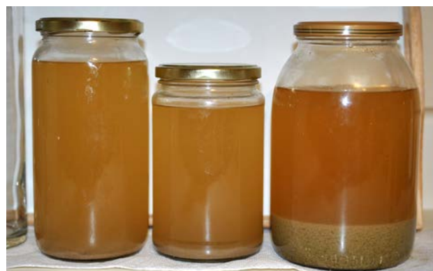
Interceptor Wastewater Samples – 24hr Settling
