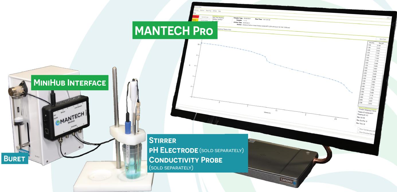
THE NEW MT5 WAS DESIGNED WITH OPERATORS FOR DRINKING WATER AND WASTEWATER TREATMENT PLANTS TO MAKE WATER QUALITY ANALYSIS SIMPLER. THE MT5 IS AN AUTOTITRATOR THAT DOES MORE – WITH THE ABILITY TO ADD MULTIPLE BURETS, CONDUCTIVITY, DO, TURBIDITY, ISE, COLOR, COD, BOD, “OPTIMIZED” TOC AND CAN BE UPGRADED TO AN AUTOSAMPLER.
