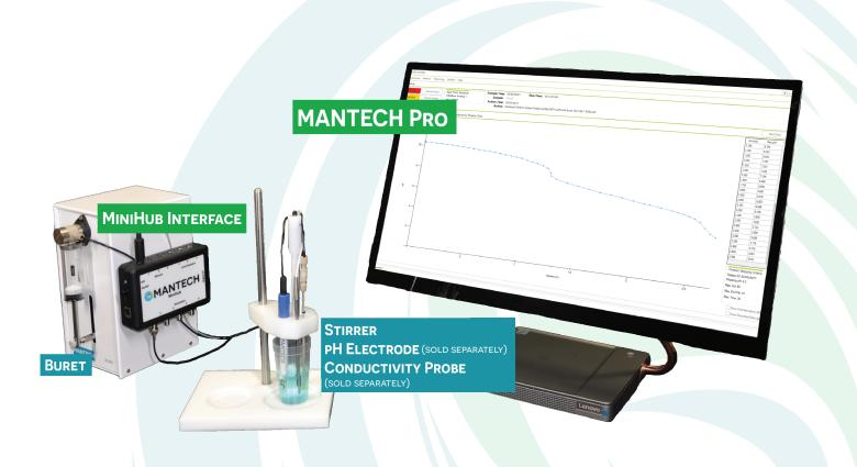
THE NEW MT5 WAS DESIGNED WITH OPERATORS FOR DRINKING WATER AND WASTEWATER TREATMENT PLANTS TO MAKE WATER QUALITY ANALYSIS SIMPLER. THE MT5 IS AN AUTOTITRATOR THAT DOES MORE – WITH THE ABILITY TO ADD MULITPLE BURETS, CONDUCTIVITY, DO, TURBIDITY, ISE, COLOR, COD, BOD, "OPTIMIZED" TOC AND CAN BE UPGRADED TO AN AUTOSAMPLER.
