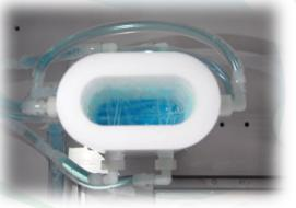
SYSTEM PICTURED MEASURES PH, CONDUCTIVITY, AND ALKALINITY FROM A SINGLE SAMPLE
