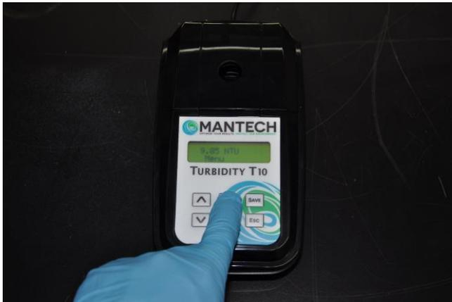
4. Press the DOWN button to show 'Calibrate' on screen, then press READ. You will see 'Guided Cal.' on screen, press READ again to start the calibration.
