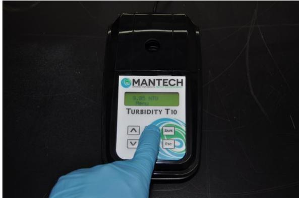
5. Press the DOWN button to show 'Calibrate' on screen, then press READ. You will see 'Guided Cal.' on screen. Press the down arrow to show 'Free Cal.' on screen instead. Press READ again to start the free calibration.
