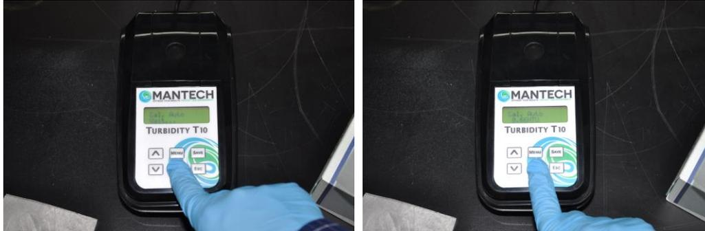
10. Use the arrow buttons to adjust the measured NTU to the expected NTU value of the standard. Hold the SAVE button for 3 seconds to save the free calibration point.
