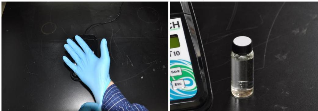
3. Prepare a Turbidity standard that is around the mid-point of expected sample results. Use the dilution chart below for preparing 40mL of various NTU standards from 100NTU stock solution:
