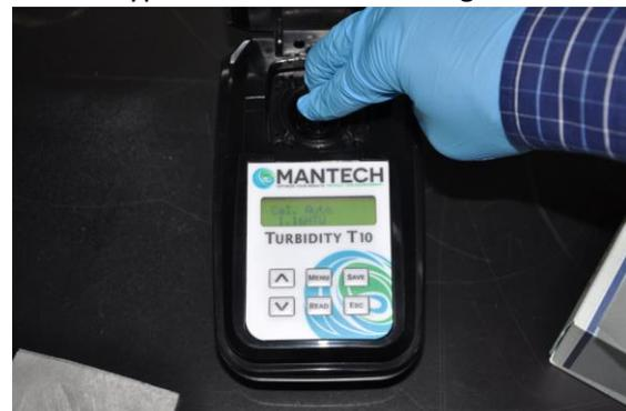
9. Press the READ button and the meter will start the measurement of the standard. You will see the measurement result appear on-screen once done.
